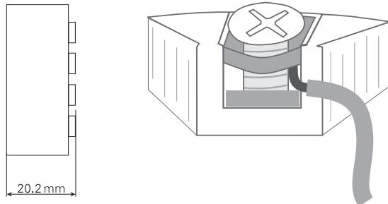
Wires must be mounted between the metal plates.
